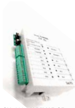
CU4200 - AUXILIAR OR OFFLINE CONTROLLER
